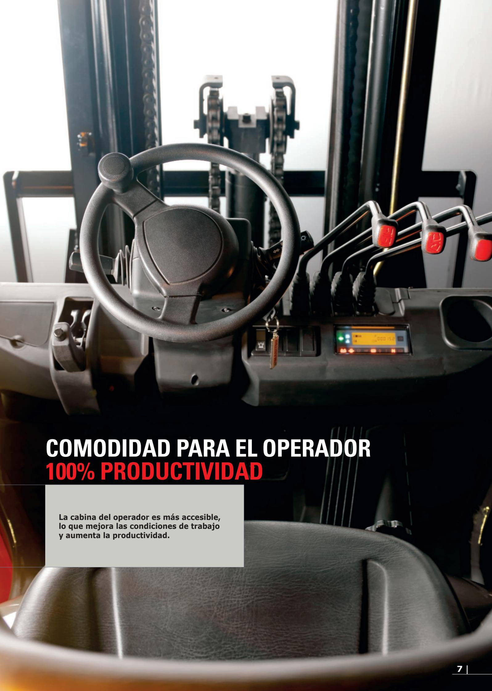
A detailed view of the operator's cab of a forklift. The steering wheel is prominent in the center, with a control panel below it featuring a digital display and several buttons. To the right, there are three levers with red safety caps. The background shows the vertical mast of the forklift. The overall lighting is bright, highlighting the metallic and plastic components of the machine.
